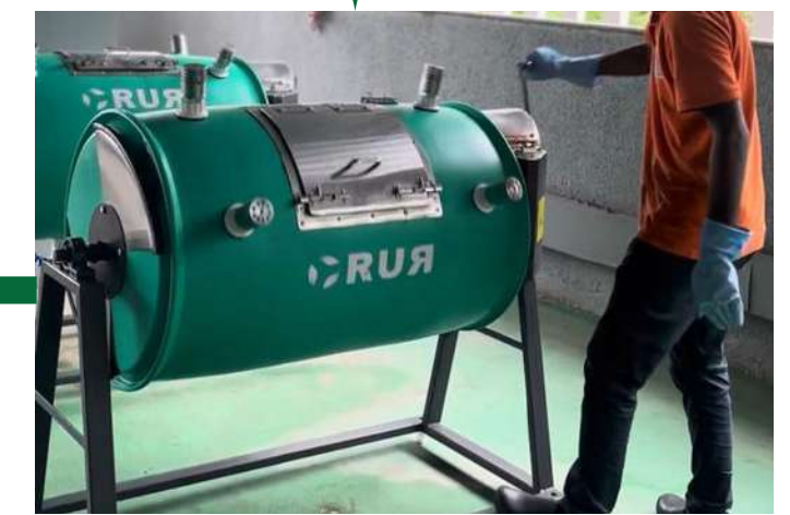
Close the drain valve and rotate the tumbler 10 times, twice weekly.
